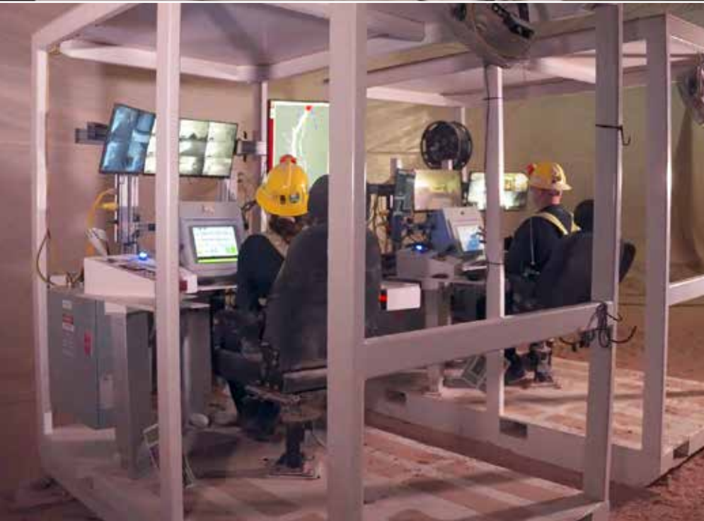
Pilot program using tele-remote technology at Nutrien Cory Mine.
